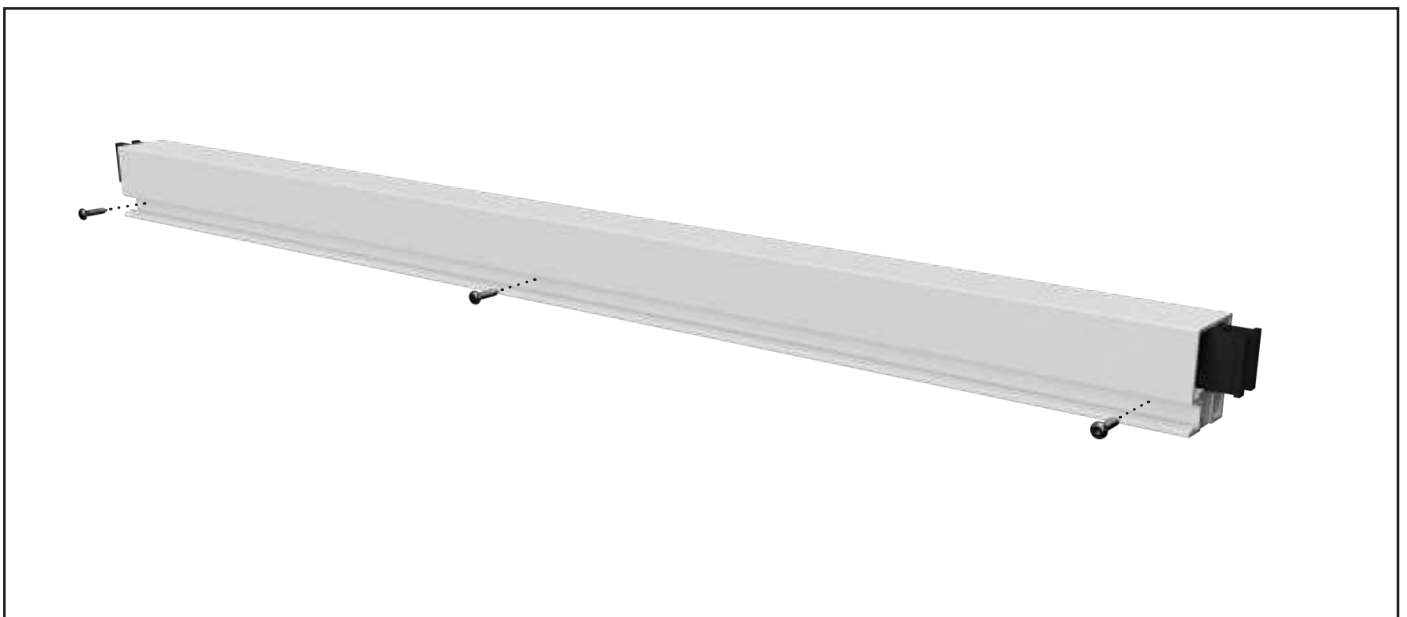
18 Secure with Gate Infill three self-drilling wafer screws within the screw channel.
