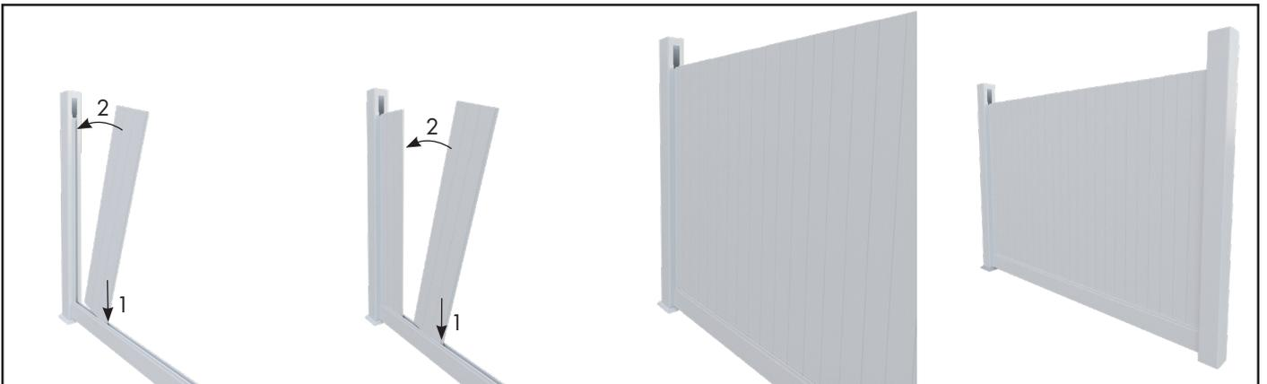
10 Starting at the vertical U channel on one side, insert vertical panels into bottom rail and lever into position. Repeat process towards the next post.
