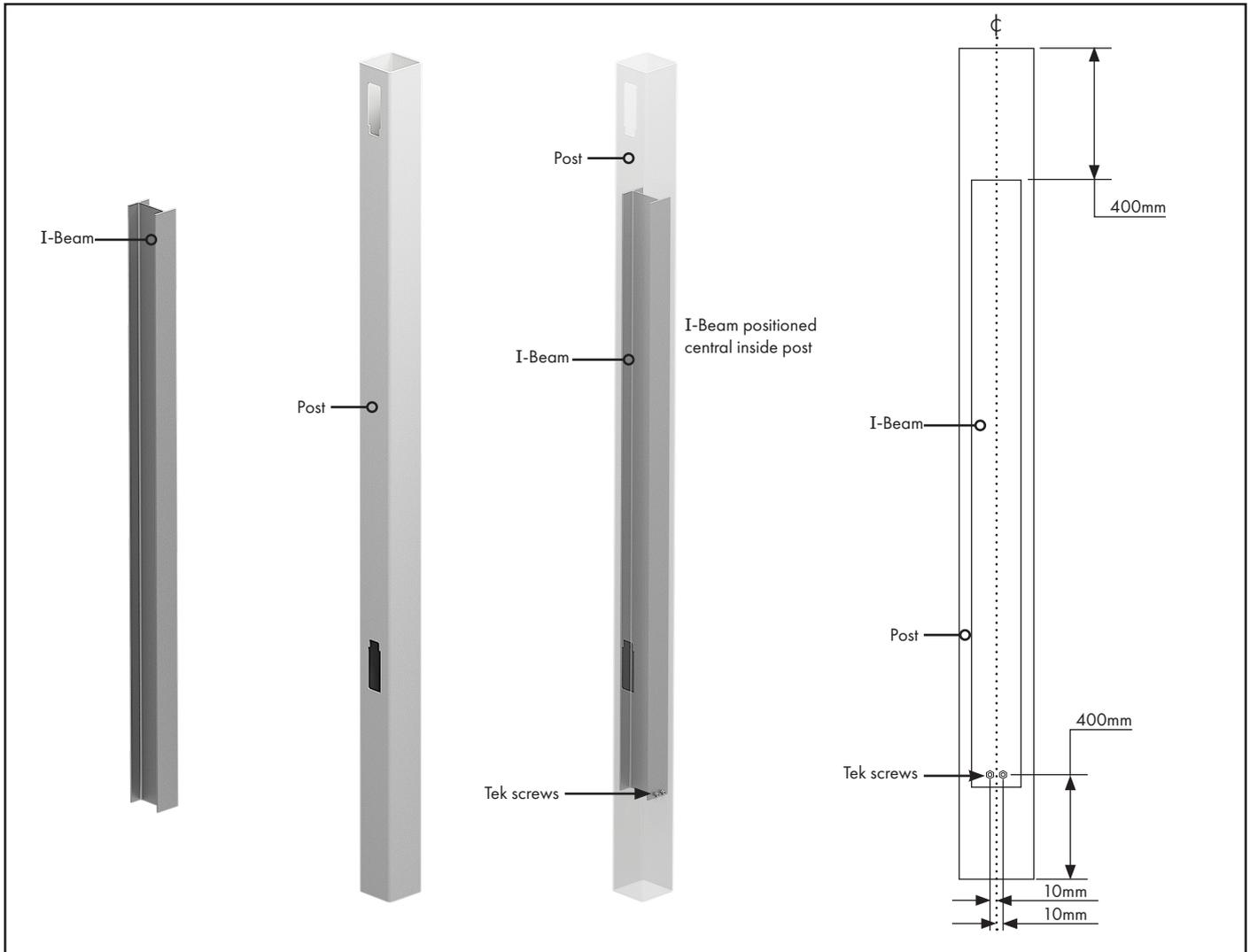
\* OPTIONAL EXTRA - ALUMINIUM INTERNAL STIFFENER I-BEAM FOR AREAS REQUIRING WIND LOAD CONSIDERATION
