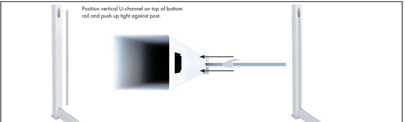
9 Position vertical U-channel on top of bottom rail and push up tight against post. Repeat step on all posts, where fence panels are to be installed.
