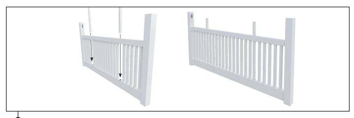
Insert long pickets through mid-rail and into bottom rail.
