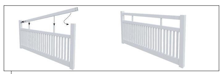
Install top rail over long pickets guiding pickets into holes on underside of top rail. Insert top rail into one post and then lever into adjacent post.
