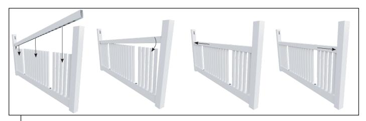
10 Push mid rail into slot on 1 post then lever into slot on adjacent post. Insert pickets as the mid-rail is levering down. Posts may flex to allow for insertion.
