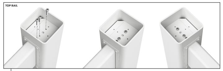
Screw top rail into place inside side frame using 3 x 25mm screws. Top plate is supplied fixed in position in side frame with holes pre-drilled for fixing through. Repeat on other side.
